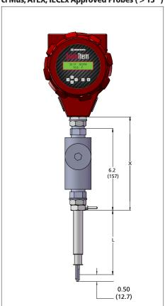
Note: All dimensions in inches with (mm) in brackets; certified drawings available upon request. All drawings have  $\pm$  .25 inch (6.4 mm) tolerance.
