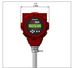
**P2-DD Compression Fitting—Side View**
